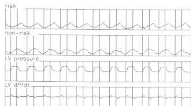
Fig. 3 Hard copy of a representative computer screen during an experiment. Digitised values of four signals, risk and non-risk wall thicknesses, LV pressure and LV dP/dt within a 3 s window are displayed. The computer-determined end-diastolic and end-systolic locations are marked with vertical lines for every heartbeat. The discontinuities during diastole in risk and non-risk signals are due to automatic resetting of the signals to prevent signal drift.
