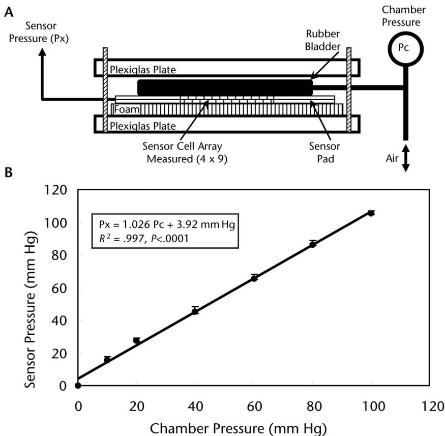
**Figure 4.** Pressure system validation. (A) Pressure system test setup. (B) Comparison of chamber pressures ( $P_c$ ) and sensor pressures ( $P_x$ ). Data points are mean  $\pm$  SD of values obtained for  $P_x$  at each independent  $P_c$  setting for all measurements obtained on 3 separate consecutive days. The solid line is the linear regression with the associated equation shown in the inset of the figure.
