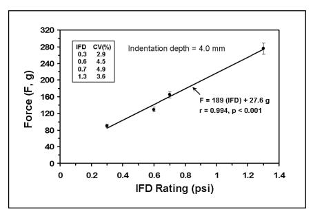
Fig. 3. Indentation Force for Polyurethane Foams. Data points show mean  $\pm$  SD of 12 indentation force trials when foam blocks with different standardized indentation force ratings (IFD) were indented to a depth of 4 mm. Inset shows coefficients of variation for force for each of the four test blocks used. Solid line is linear regression.
