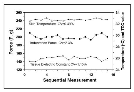
Fig. 6. Variation of Force and Tissue Dielectric Constant Measurements. Data points show sequential values of indentation force for a 4 mm indentation depth together with TDC and skin temperature values measured at 4 minute intervals on the anterior forearm of one subject. CV is the coefficient of variation over the 60 minute test period.
