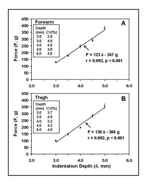
Fig. 5. Short Term Repeatability and Linearity at Different Tissue Sites. Data points show mean ± SD of 10 indentation force trials on one subject's anterior forearm and thigh. Time between repeated depth measurements at each site was 60 seconds. Results indicate a linear dependence of force with indentation depth for each site. Calculated coefficients of variation among the 10 repeated measurements at each depth are shown in the inset.
