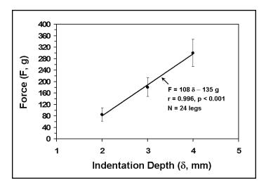
Fig. 4. Indentation Force-Depth for Healthy Legs. Data points show mean  $\pm$  SD of indentation force as a function of indentation depth for 24 legs measured at the medial gaiter area. Solid line is linear regression.
