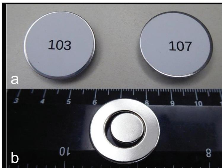
**Figure 4.** Magnet and sham devices used. (a) Magnet and sham devices used in this study visually appeared similar and had the same dimensions and weight. Each was labeled with a unique random number. (b) The Neodymium-Iron-Boron magnet had two concentric magnets, a central 12 mm diameter one within a 25.4 mm ring magnet producing a single magnetic array. The ruler in the image shows in cm.
