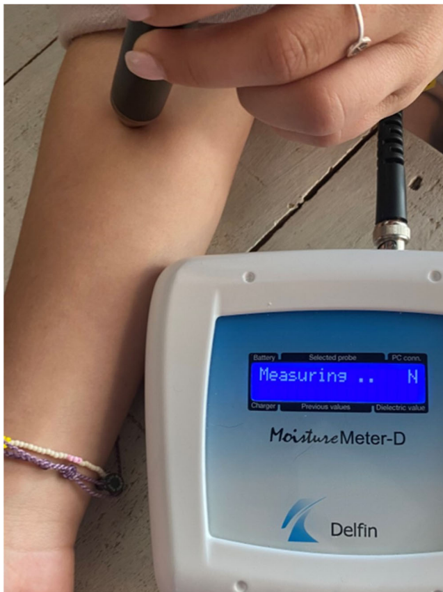
FIGURE 2 Self-measuring TDC on volar forearm. The measurement using the probe for a 0.5 mm depth is illustrated. Each depth is measured in triplicate and the average used to characterize the sites TDC value at that depth. TDC, tissue dielectric constant.
