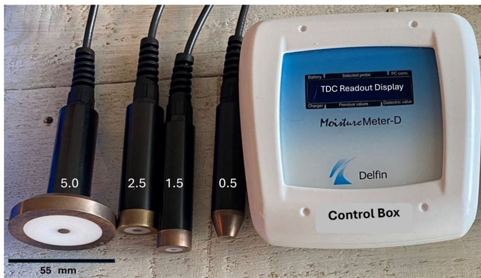
FIGURE 1 TDC measurement system. Four probes were used to measure to effective depths of 0.5, 1.5, 2.5 and 5.0 mm as labelled. Each acts as an open ended coaxial transmission line. The larger diameter allows for deeper penetration of the 300 MHz signal generated by the control box. The physical diameter of the probes from smallest to largest in mm is 55, 22, 15 and 10. Upon contact with the skin the measurement process starts and the TDC value is displayed on the readout. TDC, tissue dielectric constant.
