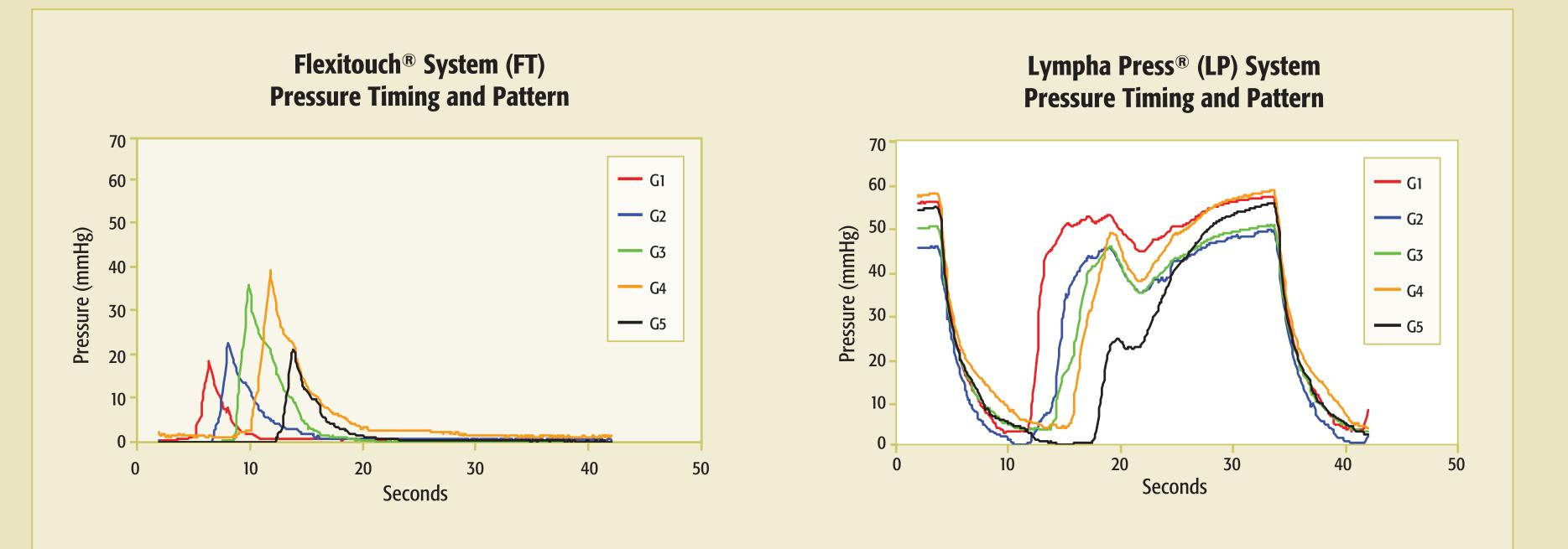
Example of temporal pressure patterns developed by the two devices. FT is crisper with a smaller peak pressure and shorter duration.
