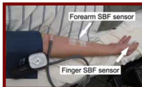
Pictured above: A TDC measurement taken by the experimenter with the arm at rest and BP cuff inflated to 50 mmHg.
